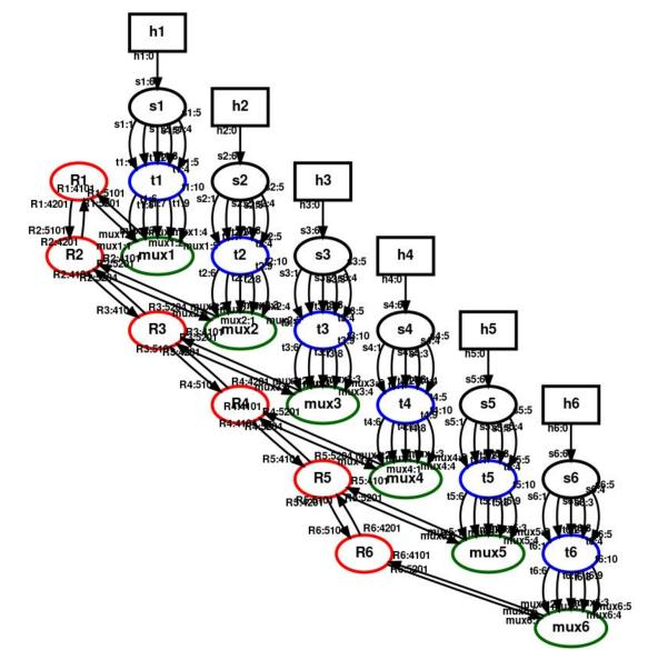
Unidirectional links; 6 split/paired ROADMs based on Lumentum; identical port numbers; comb source modeled using transceivers attached to MUX
